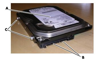
**3** Reconnect the power cable and the data cable to back of the hard drive.
